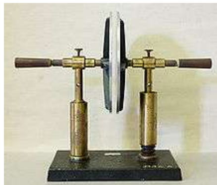
Fig 3.17: A simple demonstration of a parallel-plate capacitor
