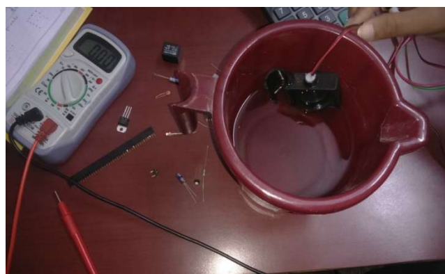
Fig 5.7: checking Magnetic float sensor
