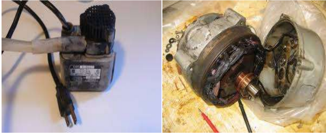
Fig 4.6: Burning out of water pump
